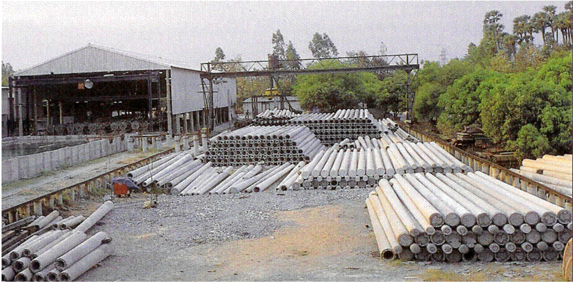
Pre-tensioned electric poles
